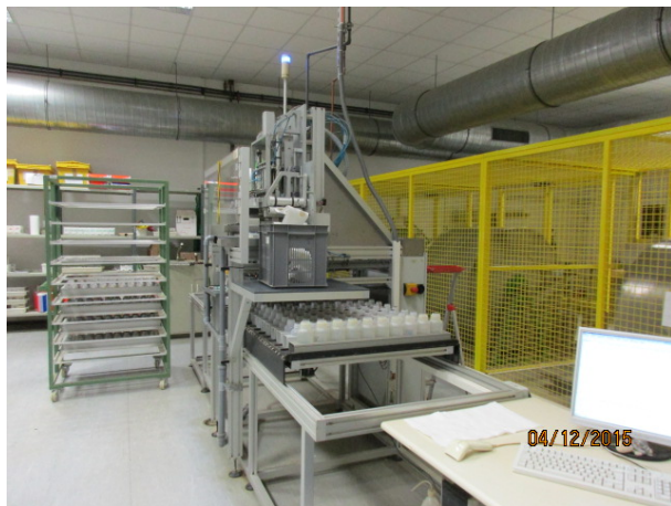
Laboratory facilities for high throughput analyses of bicarbonate extractable P at Agrolab, Germany.
