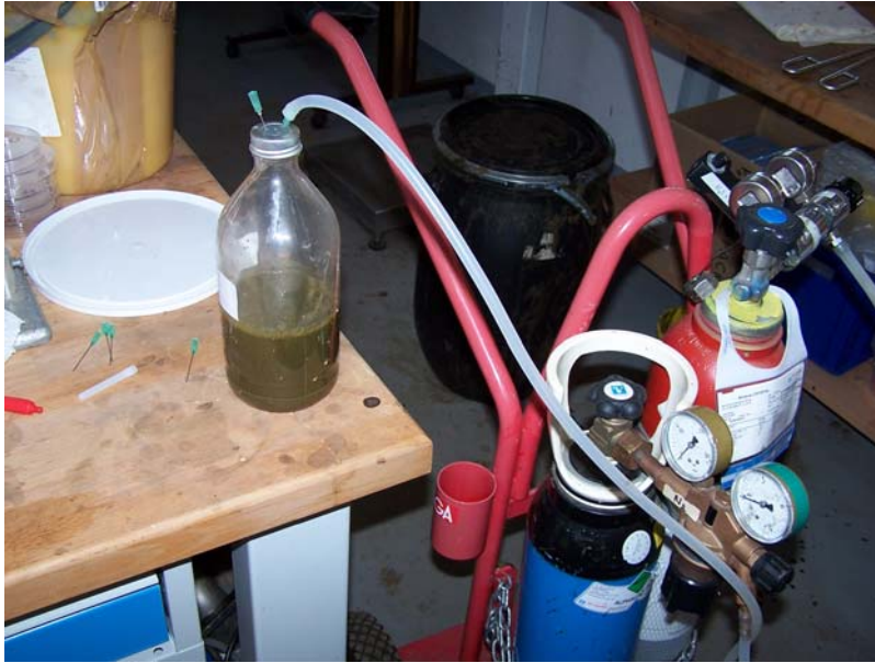
Figure 1. Nitrogen flushing of a batch test bottle to remove oxygen
