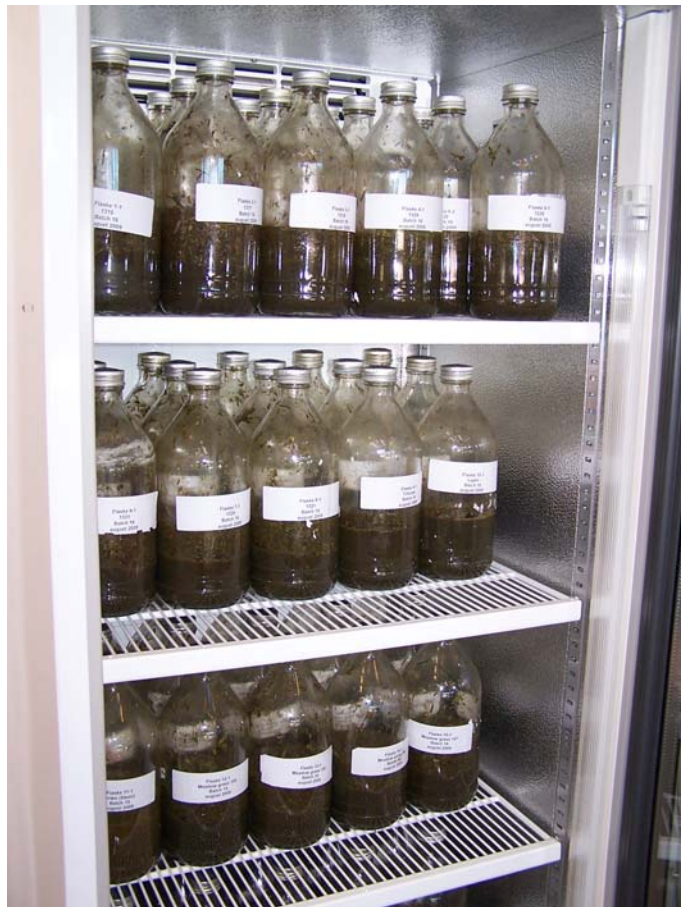
Figure 2. Batch test bottles undergoing incubation
